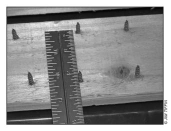
Use full or half sheets of the thickest plywood available. Nails should be long enough to stick out of the wood ¾ - 1". Nails should be nailed into the board approximately 2" apart. Drawing a grid on the board makes it easier to stay on track.
